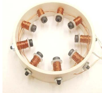
Fig. 1.a. Wound stator as it appears in the instructions.
